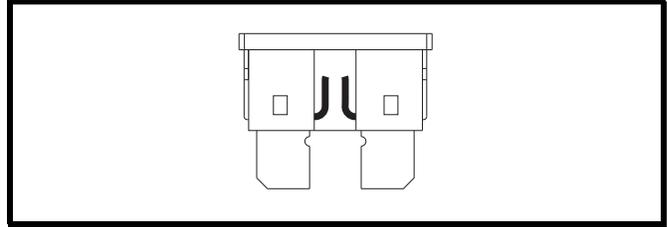
Figure 25. Blown Fuse (Replace)
