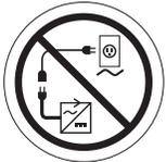
**Do not connect an extension lead to the AC/DC converter or the battery charger.**
