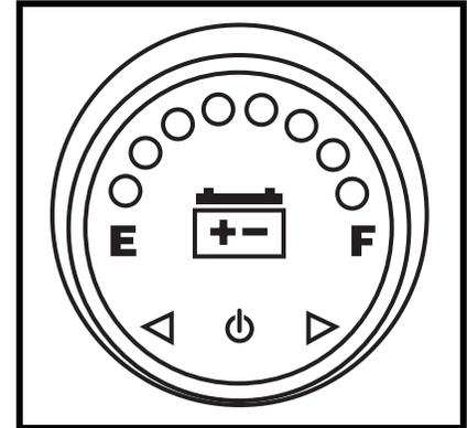
Figure 12. Battery Condition Meter
