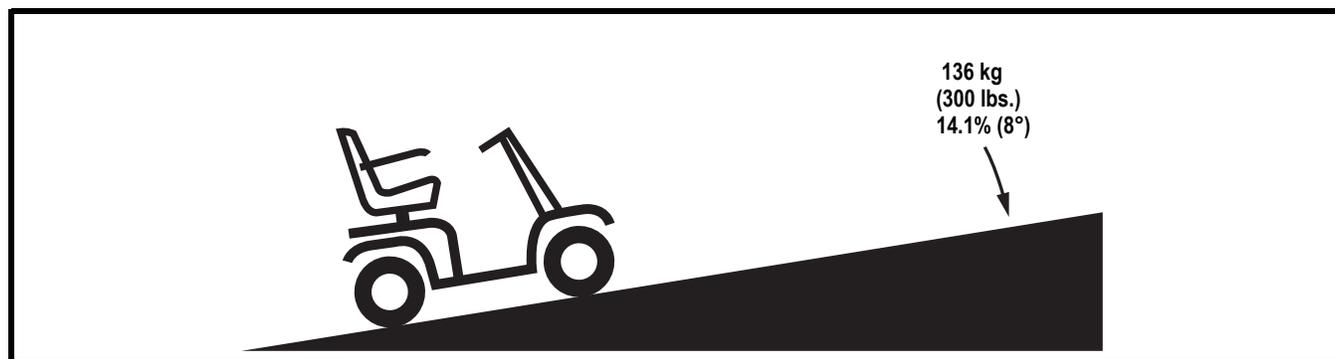
**Figure 1. Maximum Recommended Incline Angle**
