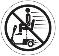
Do not raise or lower the power seat while the scooter is in motion.
