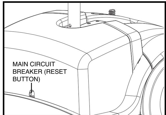
**Figure 8. Main Circuit Breaker (Rear Section Mounted)**
