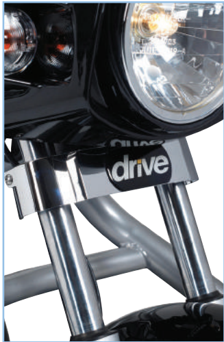
Telescopic front motorcycle suspension for optimal handling
